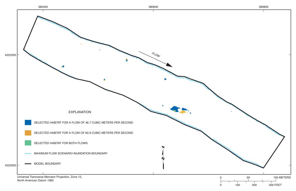
Figure 5-96. Selected habitat area distribution for habitat categories 24, 25 combined (stonecat) at flows of 46.7 and 60.9 cubic meters per second at Marais des Cygnes River site MDC3.
